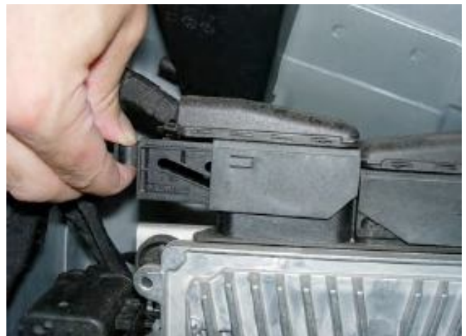
Disconnect the small connector by pulling the release tab as shown above
